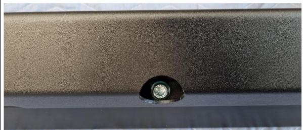
19. Fit the step onto the slider extrusion.
